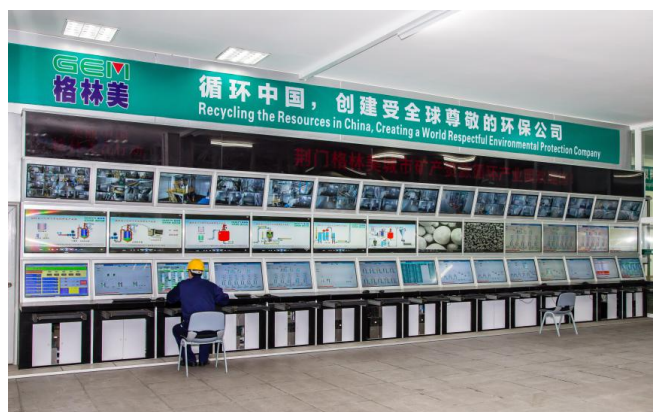
Figure 5. The automatic control system of GEM power battery precursor material production line. [Photo courtesy of GEM Co., kindly reproduced from gem.com.cn ].
