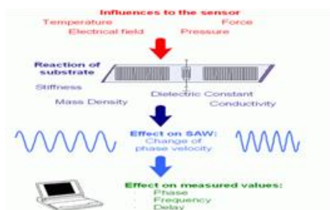
Figure 5 - Shape of the signal across the sensor
