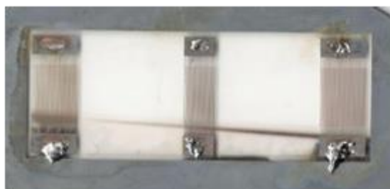
Figure 15 - Produced dual-channel delay line
