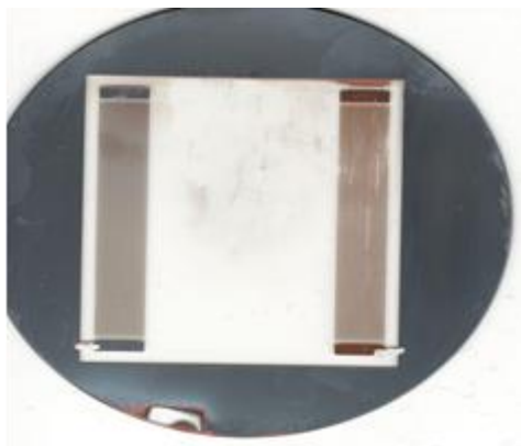
Figure 10: The process metallization by putting copper and vanadium and etching this by laser appellation as shown in [3]
