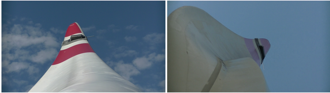
Figure 6. View from the optical camera on the spinner to the pressure side of the blade at R = 35 m. The black box contains all the data recording system including power supply. Chord there is 1.5 m. In addition, orientation of the 5-hole-probe relative to vertical axis (approx. rotor plane) indicates the instantaneous pitch to be compared with values from the SCADA system. Left: WT in standstill, right: WT in operation.
