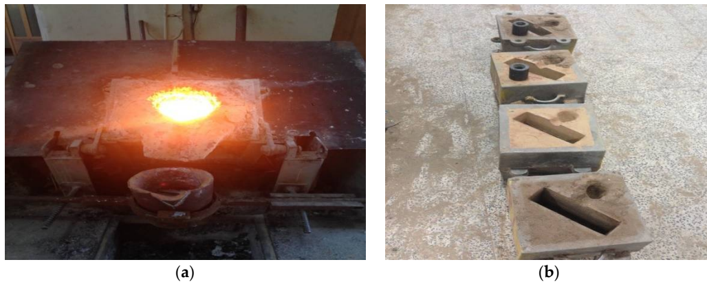
Figure 1. Induction furnace; 1 b. Sand mold.
