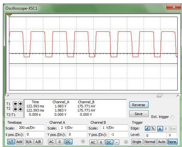
Figure 4. The output voltage at the frequency of 4.0kHz and Csensor of 1nF.
