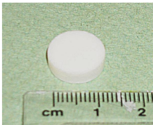
Figure 1. Freeze-dried powders were compressed to produce BCG-loaded Eudragit matrices of 13 mm diameter and 2.2 mm thickness.
