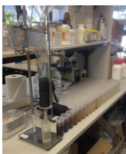
Figure 3: Setup for the column leaching tests (note the improving clarity of the eluted samples)
