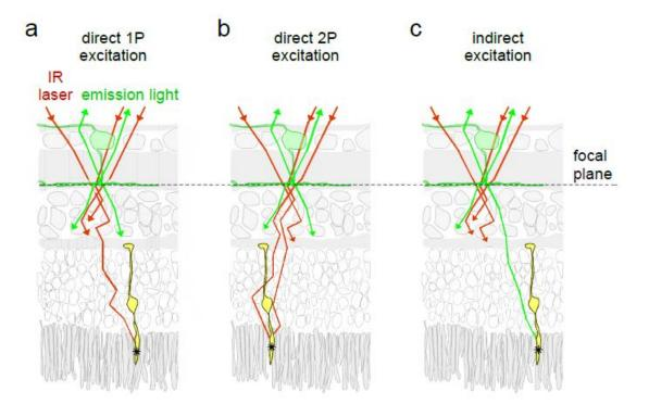
Fig. 2. Direct and indirect excitation of PRs
