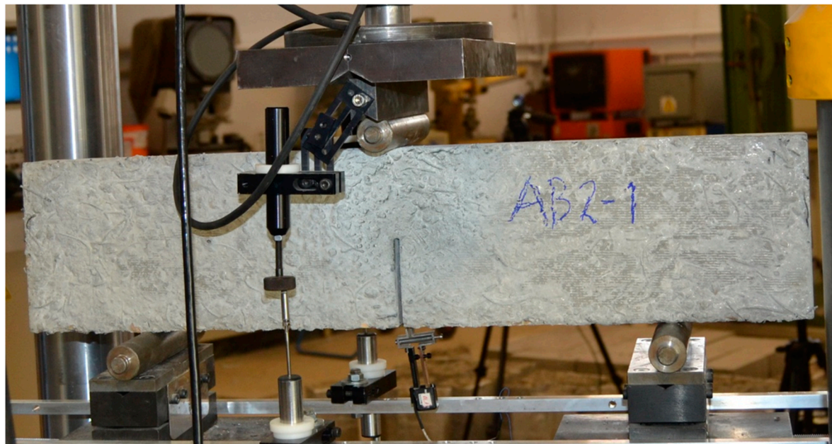
Figure 4. Beam specimen ready for testing.
