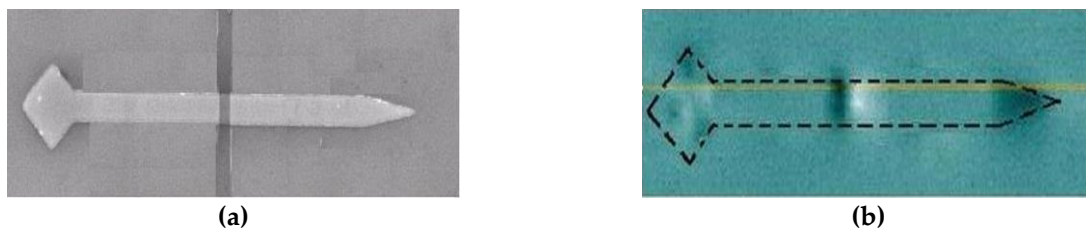
Figure 2. (a). SEM picture of the diamond-stripe series wire and (b) The MFM images of the device. The dash line is the guide line for the wire.
