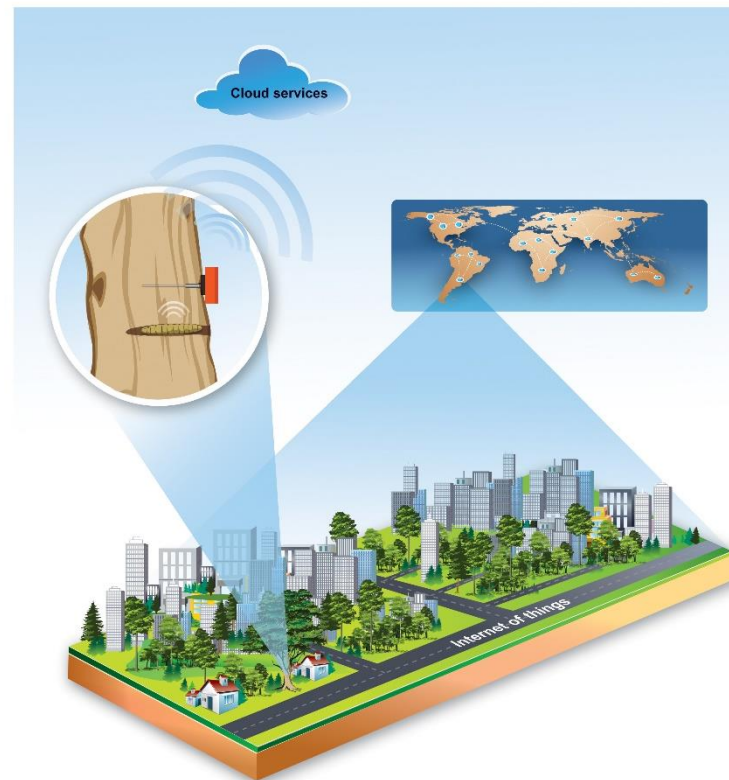
Figure 1. The concept of in-vivo acoustic surveillance of trees in forests and urban environments. Trees are probed for real-time monitoring against wood-boring insects. The device emits recordings of vibrations stemming from inside the tree trunk due to feeding or moving sounds of larvae. The IoT expands the remote monitoring application from a few trees to regional, national or global networks.
