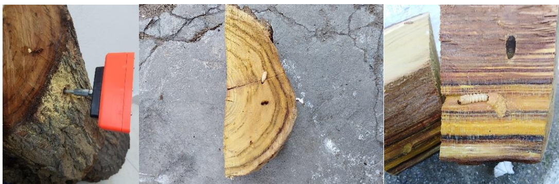
Figure 9. A X. chinensis positive case in a mulberry trunk. (left) The sensor mounted horizontally in a suspicious trunk in the laboratory, (middle and right) two alive larvae have been found after cutting the suspicious trunk in slices. The larvae tunnels can be seen in the right picture.
