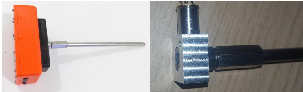
Figure 2. (left) The vibrations recorder: a rugged container for outdoor deployment contains the electronics including GPS and GPRS, (right). Detail of the metal waveguide fastened to the input of the accelerometer. The tree trunk is first drilled using a bit matching the size of the probe and the waveguide is subsequently inserted and fastened in the hole.
