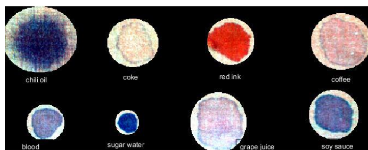
Fig.10. the hyper-spectral image of stains on red T-shirt after preprocessing and ROI extraction.
