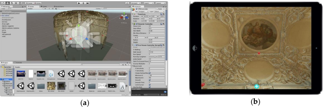
Figure 24. (a) Arranging camera position inside the 3D textured model using FirstPersonController of Unity. (b) Interactive model of the hall showing typical points enabling to reach additional information.
