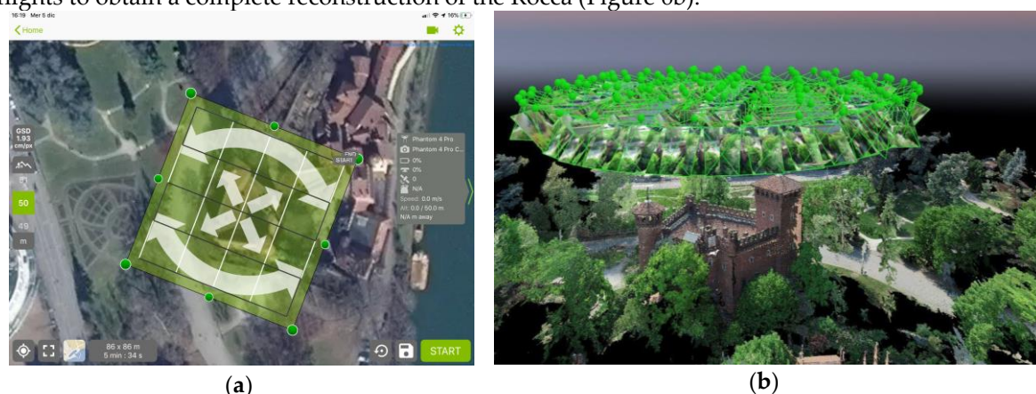
Figure 6. (a) The flights performed by Phantom 4 PRO (b) oriented UAV images block on the Rocca
