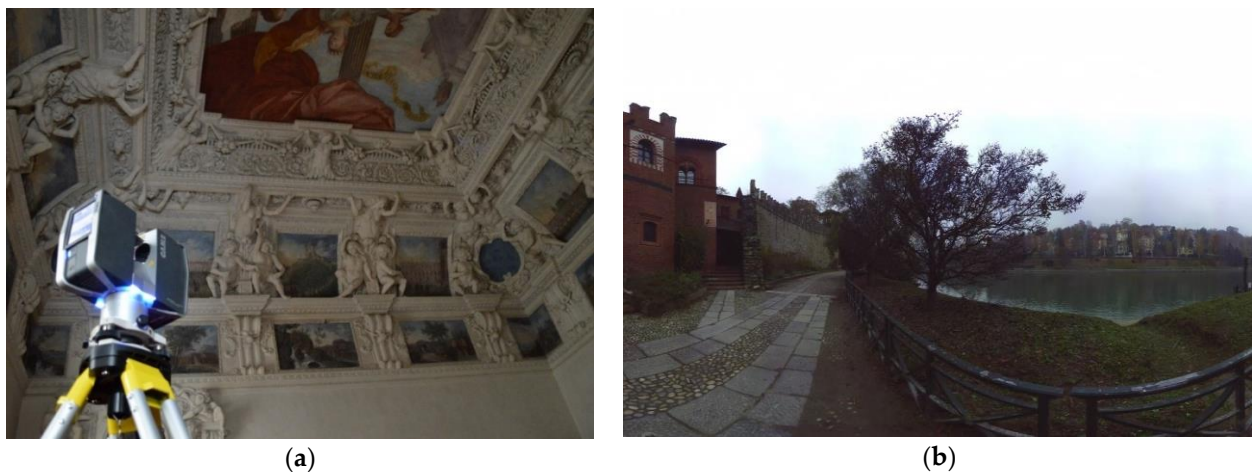
Figure 3. TLS by Faro: (a) The FARO Focus 120 during the acquisition and (b) planimetric view of an outdoor coverage range of an X330 scanner
