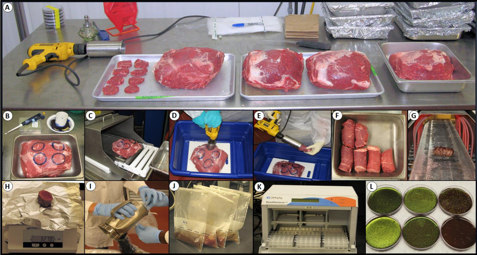
Figure 2. Phase 2, evaluation of select antimicrobials against E. coli O157:H7-inoculated beef subprimals in conjunction with blade tenderization. (a) array of beef subprimals during one trial; (b) beef subprimal prepared for inoculation in labeled zones; (c) inoculated beef subprimal entering blade tenderizer; (d) sprayed and blade-tenderized subprimal being cored; (e) recovery of beef cores using 2-inch circular drill bit; (f) recovered beef cores; (g) sanitizing outside of beef cores by passage through radiant heat oven; (h) sectioning of beef cores; (i) blending and (j) enrichment incubation of beef sections; (k) Bead Retriever™ for immunomagnetic bead recovery and enrichment of E. coli O157:H7 from enrichment broth; (l) plating of immunomagnetic beads with recovered E. coli O157:H7 onto EMB media containing rifamycin.
