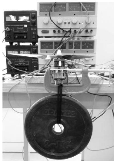
Figure 3. Experimental setup to characterize the motor thrust.
