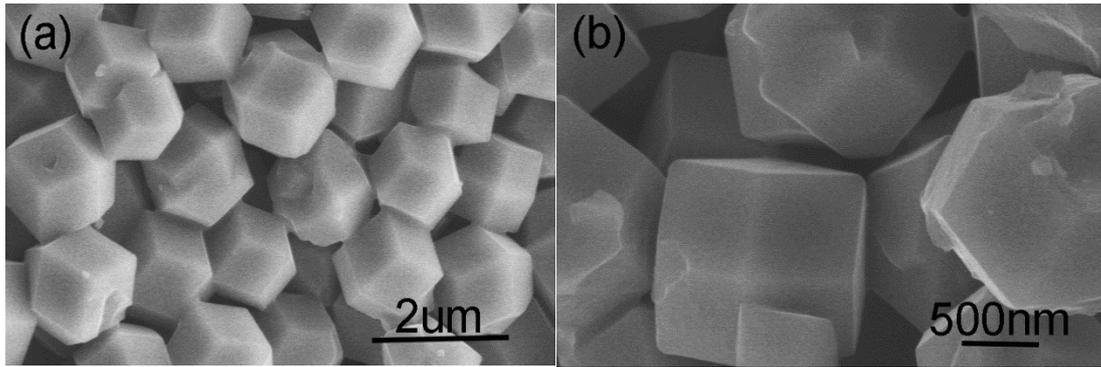
Fig. S2 The Low-(a) and High-magnification (b) SEM images of the synthesized ZIF-8 without CTAB.
