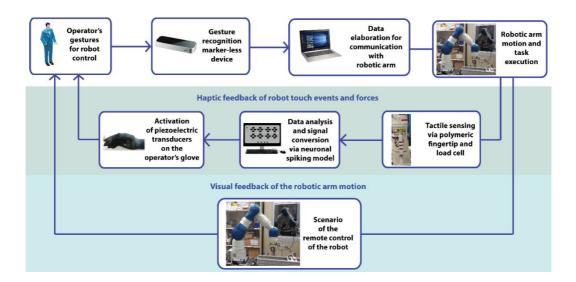
**Figure 1. Block diagram of the robotic arm with bidirectional gesture control system.** The hand movements of the operator are recognized by means of marker-less infrared stereo camera and delivered to the robot as motion commands while the operator is fed back with spiking vibrotactile stimuli representing the commanded robot velocity and its tactile interaction with the environment.
