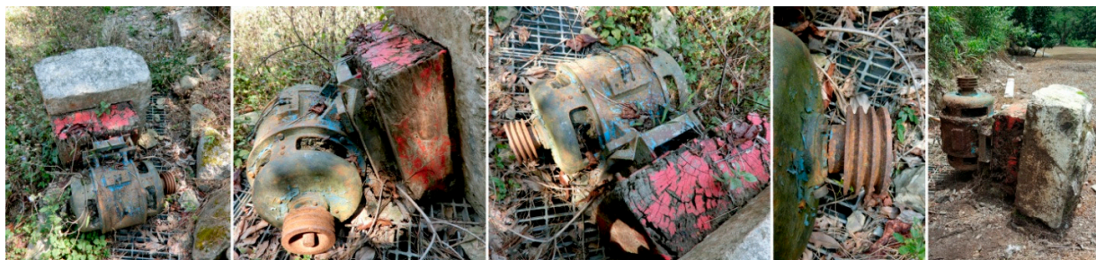
Fig. 13. Electric generator, the last picture shows that the data plate is already rusted. (Source - Author)
