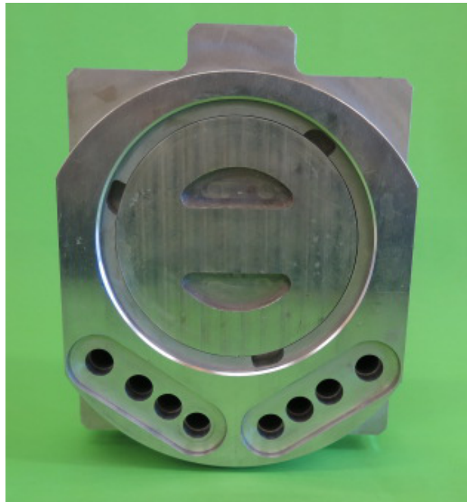
Figure 8. A closed tandem target holder with the bayonet-mount plug in position.
