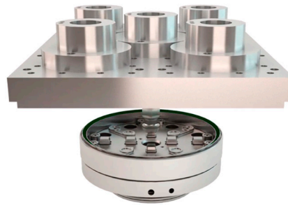
Figure 10. 3R tooling system used for keeping a fixed reference during the whole process [112].
