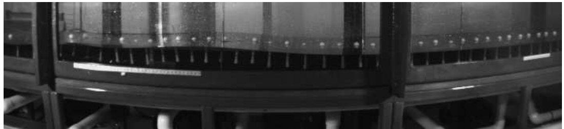
Figure 3: Gravity wave passing through the middle of the one-dimensional buoy chain. The water wave has amplitude 0.12cm and wavelength \lambda = 1.6m . The nonlinear wave initiated in the magnetic chain has already arrived at the far right end.
