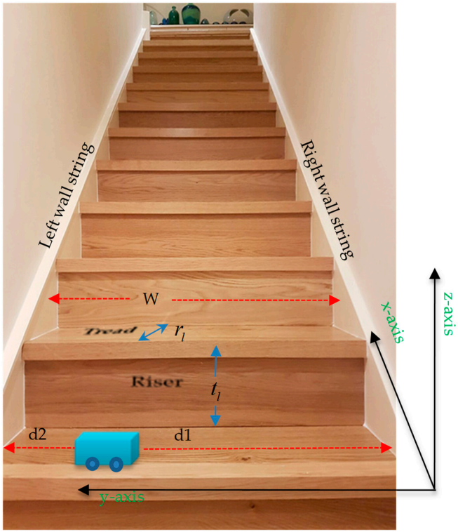
Figure 2. Staircase geometry to calculate 3D position and orientation of sTetro robot.
