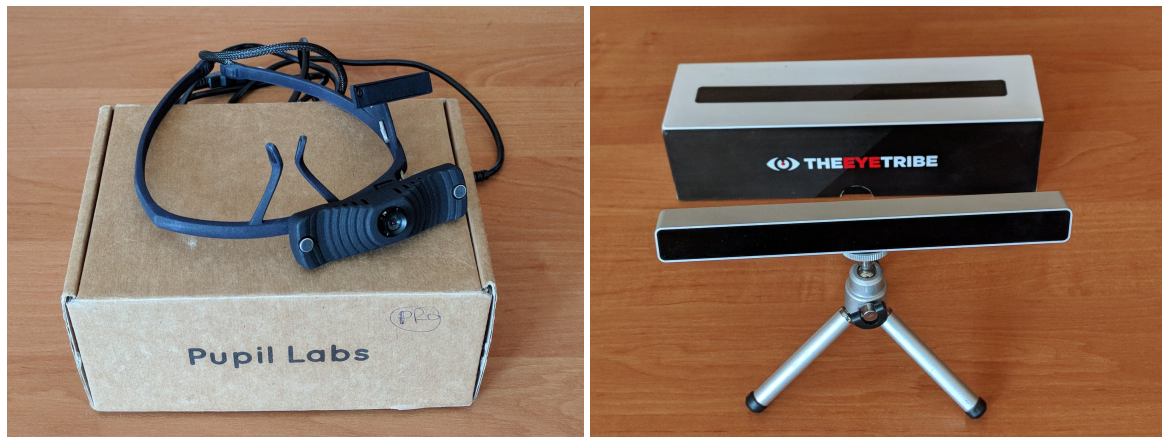
Figure 5. Eye trackers used during the experimental part of the research. Left: Pupil Labs head-set eye tracker, right: The Eye Tribe remote eye tracker to be mounted below a screen.
