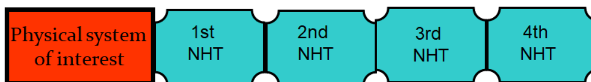
Figure 1. Schematic representation of the NHC method and its operating. The temperature of the physical system (red box) is controlled by the mechanism of the NHC equations (all four green boxes). That is, the first Nosé-Hoover thermostat (1 st NHT) in the chain is coupled to the physical system, the second (2 nd NHT) is coupled to the first Nosé-Hoover, the third (3 rd NHT) is coupled to the second thermostat, the (4 th NHT) is coupled to the third thermostat Nosé-Hoover, and so on, until forming a collective system of Nosé-Hoover chains (NHC).
