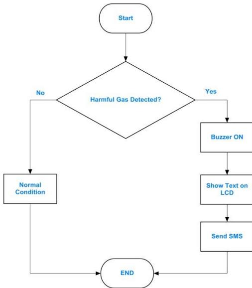
Figure 6: Flow chart of harmful gas detection section.
