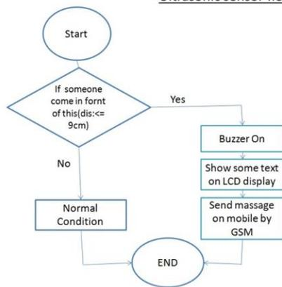
Figure 7: Flow chart of intruder’s detection mechanism.
