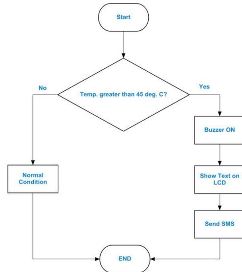
Figure 5: Flow chart of temperature detection system.
