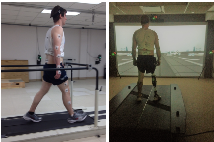
Figure 3. Experimental setup for data collection. The left figure shows an able-bodied subject and the right figure shows an amputee subject with an Ottobock prosthesis on the right leg.
