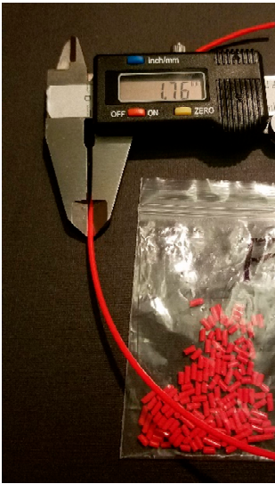
Figure 15. Example filament with a diameter of 1.75mm +/- 0.10mm made from RepRapable recyclebot from pelletized filament shown in bag.
