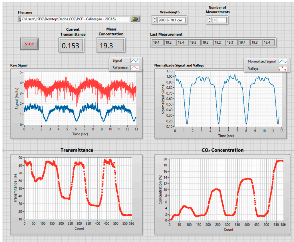
Figure 5. Computer interface of the acquisition and processing unit of the sensor
