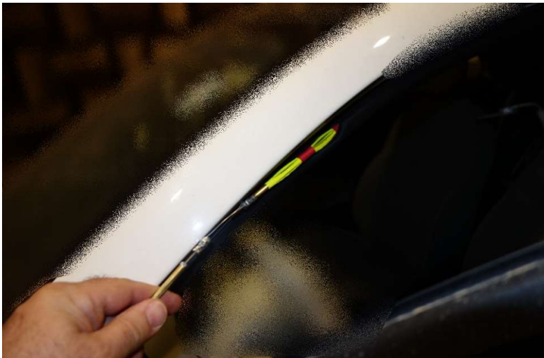
Figure 21. Integration of the SMA adaptive system within the door seal.
