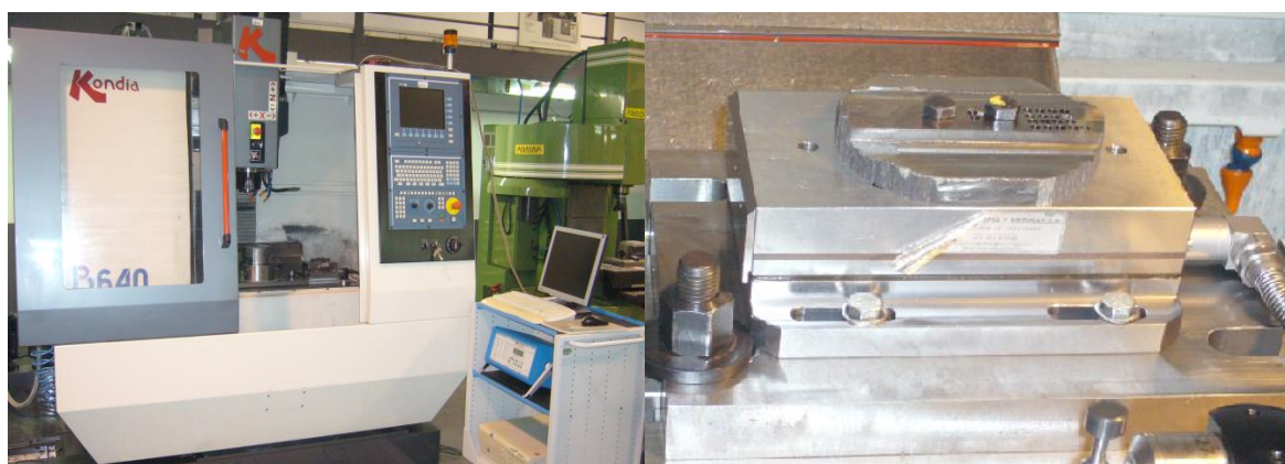
98 Figure 1. Kondia® model B640 (left) and Kistler® 9257B dynamometer (right)
