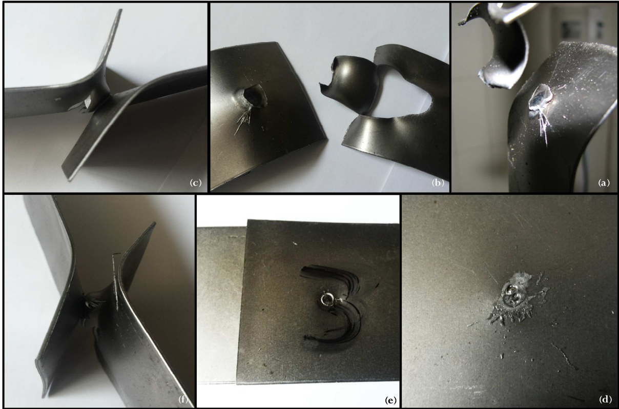
Fig. 9. The peeling test and final results.
