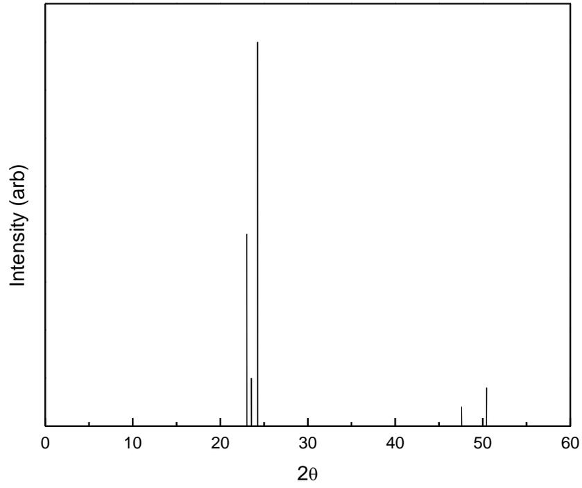
**Figure S1.** XRD pattern of WO<sub>3</sub> Film
