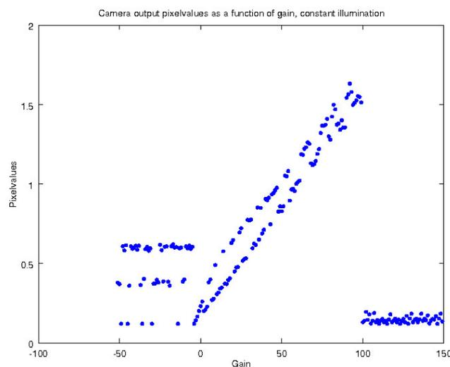
**Figure 1.** Camera output pixelvalues as a function of control gain SDK parameter under constant illumination. We see that negative values and values over 99 do not result in linear gain control.
