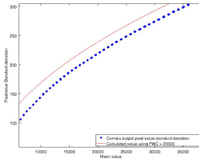
**Figure 3.** Camera output pixel value standard deviation as a function of mean pixel value under constant illumination. The calculated curve indicates that the equivalent full well capacity (FWC) is close to 23000.
