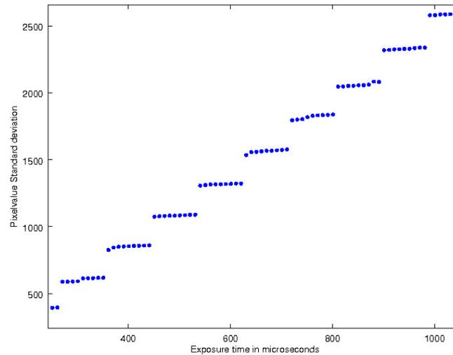
**Figure 2.** Camera output pixel value standard deviation as a function of CONTROL\_EXPOSURE SDK parameter under constant illumination. The step function response indicates that the actual exposure time varies only in steps of around 100 microseconds.
