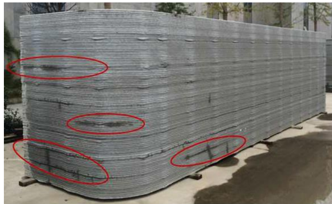
Figure 1: Signs of pronounced local water-intake (highlighted) at the layer interfaces, presumably due to high porosity of the interlayer, photo by V. Mechtcherine
