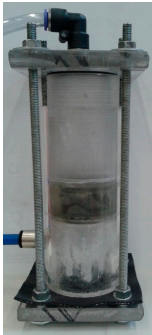
Fig. 4. Gas permeability meter: a) view, b) construction scheme:
