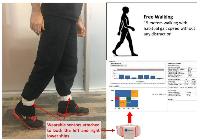
129 **Figure 1.** An Illustration of gait test. Two wearable sensors were attached to left and right lower shins.
