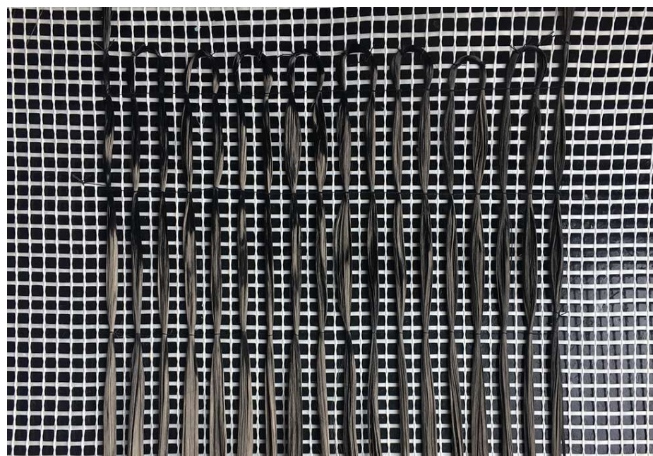
Figure 2. The third generation of textile sensor during fabrication.
