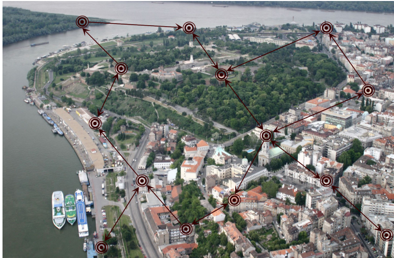
Figure 1. An example sensor network used in smart-city applications with decentralized communication topology. The inter-node communication is performed according to the depicted directed graph. The introduced distributed calibration algorithm achieves asymptotic calibration of all the sensor nodes in the network without using any type of fusion center.
