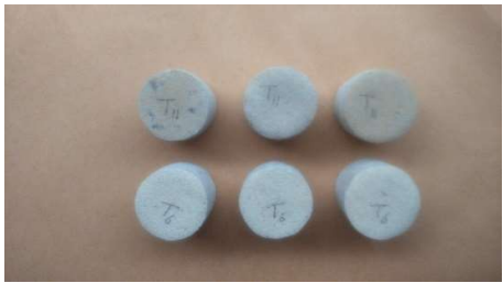
Figure 7. Synthesized Composites as Samples Made of Activated Zeolite, Banana Stem Fibre and Binder (PVAc and CaO)
