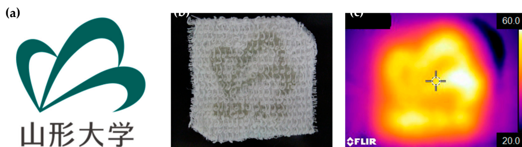
Figure 10. The logo of Yamagata University (a), the printed logo on cotton fabric using P(SA-DMAA) gel (3DP 0.25) as printing material on LumiForge (b), and its infrared thermal picture supplied by an infrared thermal graphic camera (c).
