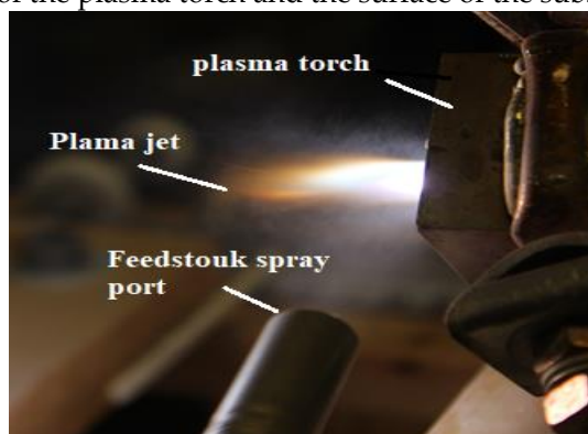
Fig. 5 Appearance of the external feedstouk sprat to the plasma jet.
