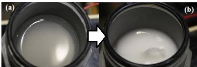
Fig. 3 Appearance of the suspension particles located at the bottom of the container (a) before agitate the suspended particles and (b) after agitate suspended particles using ultrasonic waves.
