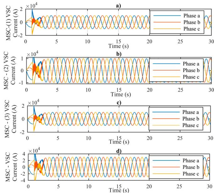
**Figure 6** Current present in MSC of AFE parallel converter. a) (1) VSC; b) (2) VSC; c) (3) VSC; d) Total current.
