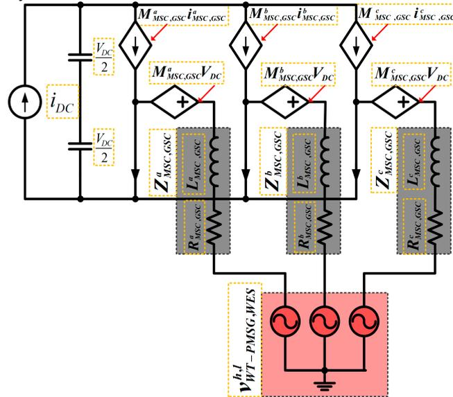
Figure 4 Three-phase VSC equivalent circuit
