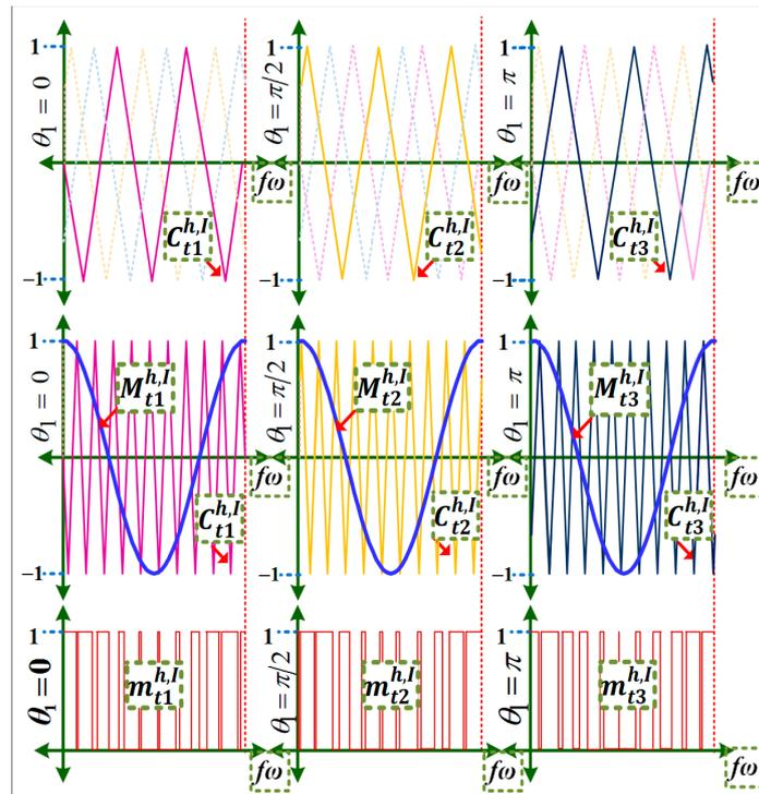
Figure 3 DSPWM signal applied to each VSC connected in parallel (phase a).
