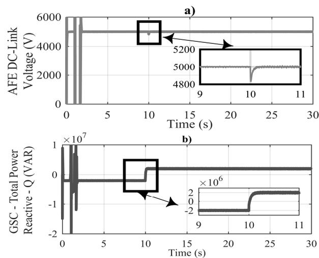
**Figure 7** DC-Link and Reactive Power controlled by the GSC. a) DC-link voltage; b) Exchange of reactive power in WES.
