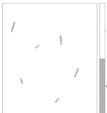
Figure 11. Spatial distribution of detected vessels based on maximum likelihood classifier (MLC) method, where gray color with zero value stands for the locations of detected vessels and the white color with the number 1 corresponds to the non-vessel pixels representing ocean pixel.
