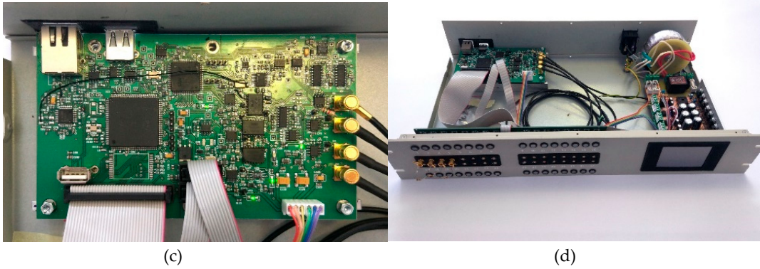
Figure 19. Hybrid tomography scanner: (a) measuring block, (b) control and communication system, (c) view from the inside, (d) measuring panel
