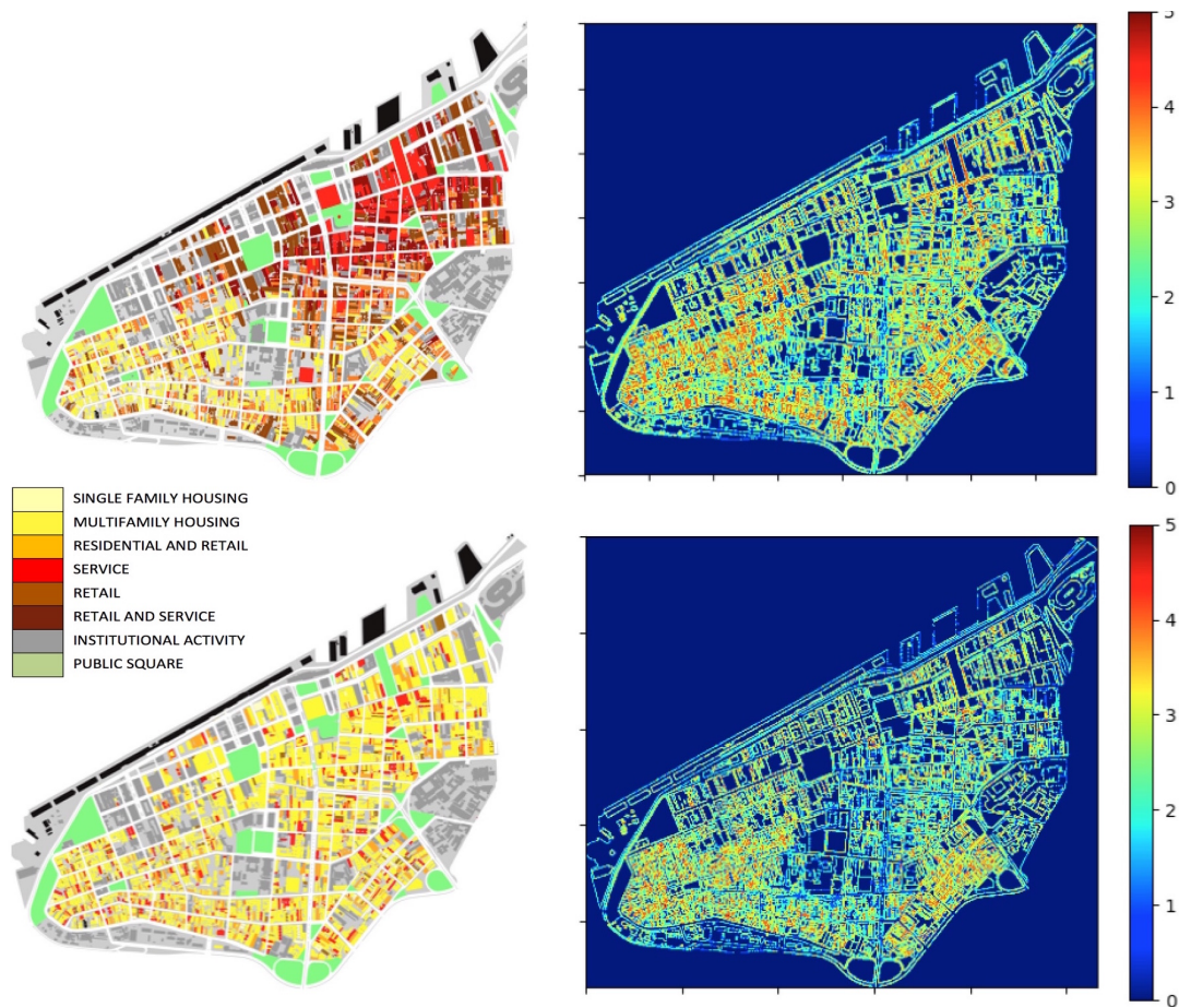
Figure 8. Semantic maps: real distribution (top) and fictitious distribution (bottom) of land uses in Porto Alegre's CBD, Brazil on. Corresponding H_j^m values are shown on the right. Entropy values shown on the right (from blue to red) are calculated with equation 3. Values are calculated for m = 10 , with the cell j corresponding to a pixel of the maps on the left. The calculation is run over a gray-scale copy of the maps. Source: Authors based on [77].
