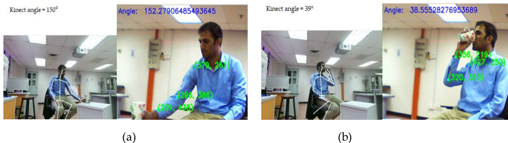
Figure-4. Shows angle estimation in two different static poses by RGB camera and Ms Kinect. The angle in black color on left side of both (a) and (b) is of Ms Kinect and angle in blue color is of RGB camera.
