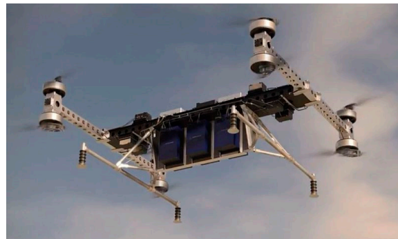
Figure 13. The Boeing HorizonX is an unconventional eVTOL cargo air vehicle [71]
