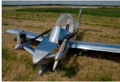
Figure 14. Cri-Cri, the World smallest twin engine manned aircraft designed by French Colomban ( https://en.wikipedia.org/wiki/Colomban_Cri-cri )
