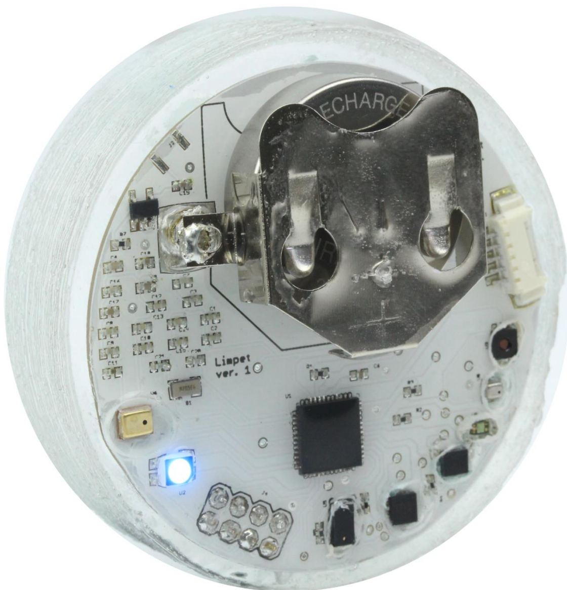
Figure S2: A picture of a Limpet in a protective housing made of clear polyurethane resin.
