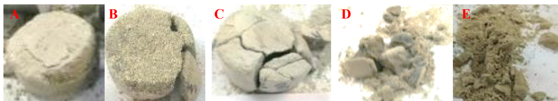
Fig 10. Failure forms and destroy degree of CPB specimens Group 70-6-90. (A) NO. 70-6-90-1, it almost had no destruction and kept as a whole and completeness under a low impact velocity 3.68 \text{ m}\cdot\text{s}^{-1} ; (B) NO. 70-6-90-2, still kept as a whole, but began to break from the peripheral and occurred a few fine cracks under an impact velocity 4.69 \text{ m}\cdot\text{s}^{-1} ; (C) NO. 70-6-90-3, be split to parts along main cracks which resulted in perforation failure under an impact velocity 5.10 \text{ m}\cdot\text{s}^{-1} , but still kept little residual strength; (D) NO. 70-6-90-4, be crushed to many
