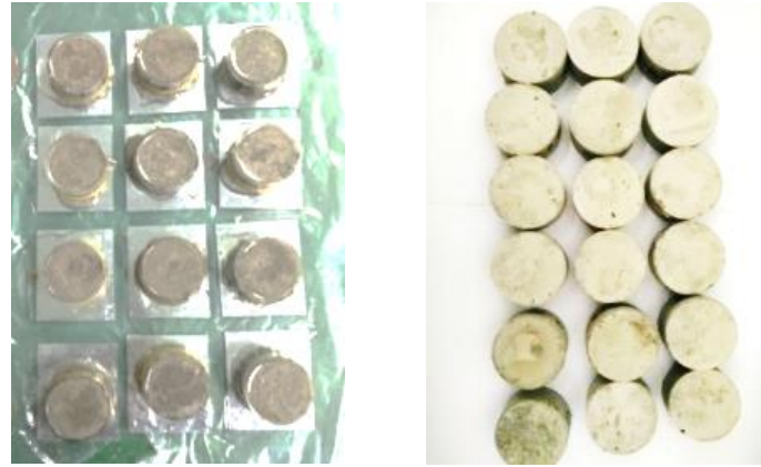
Fig 2. CPB specimens made by slurry mixed by classified tailings, 425# portland-cement and water with cement-sand ratio of 1:4, 1:6, 1:8 and concentration of 70% and 75%. They were classified into 6 groups by cement-sand ratio and concentration (Group 70-4-90, Group 75-4-90, Group 70-6-90, Group 75-6-90, Group 70-8-90, Group 75-8-90). Group number represents the corresponding parameters of CPB specimens. For example, Group 70-4-90 means the slurry concentration is 70%, the cement-sand ratio is 1:4 and the maintenance time is 90d. while in below, 70-4-90-1 represents the No. 1 specimen of the Group 70-4-90.
