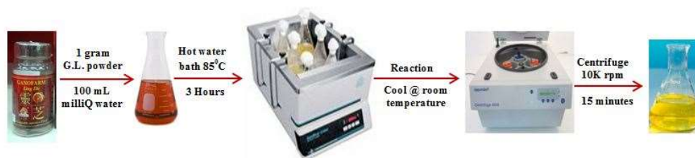
Figure 2. Schematic illustration of preparing Ganoderma lucidum extract.
